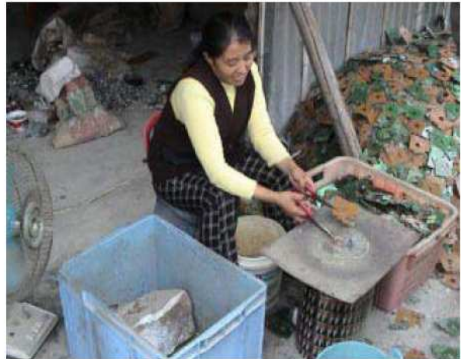
Laborer de-soldering circuit boards over a coal-fired grill. Rock in the box is where boards are hit to remove solder. Pliers are used to pluck off chips which go into various buckets. The boards are then tossed into a pile for open burning. © BAN
